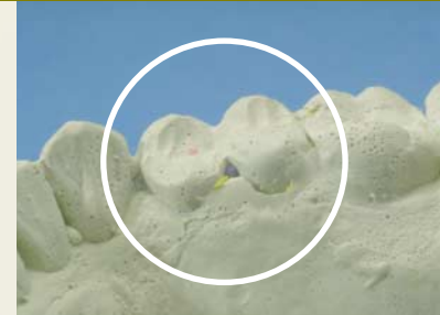
Stone model with hydrogen evolution voids
